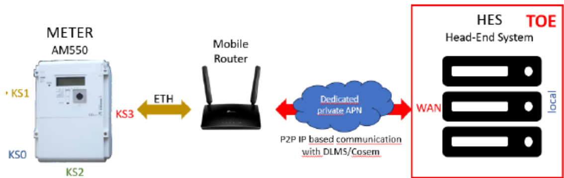
Fig. 2 – Schematic picture of complete intelligent Measuring System (iMS) with iMS component SEP2W-HES (P2P connection via mobile router)
