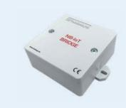
The Holosys NB-IoT PulseReader P1N is a communication module used for remote reading of energy consumption (gas, electricity, heat) and water. The module collects readings from the pulse outputs of meters of various manufacturers and transmits them to the NB-IoT telecommunications network.
